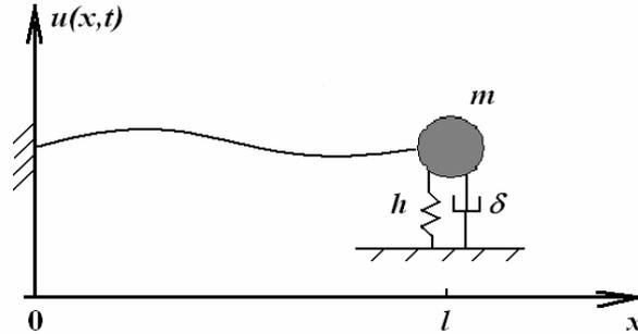
Figure 1.- Scheme of model I
