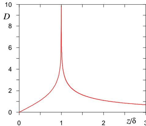
Figure 2.- The logarithmic decrement as a function of the impedances ratio
