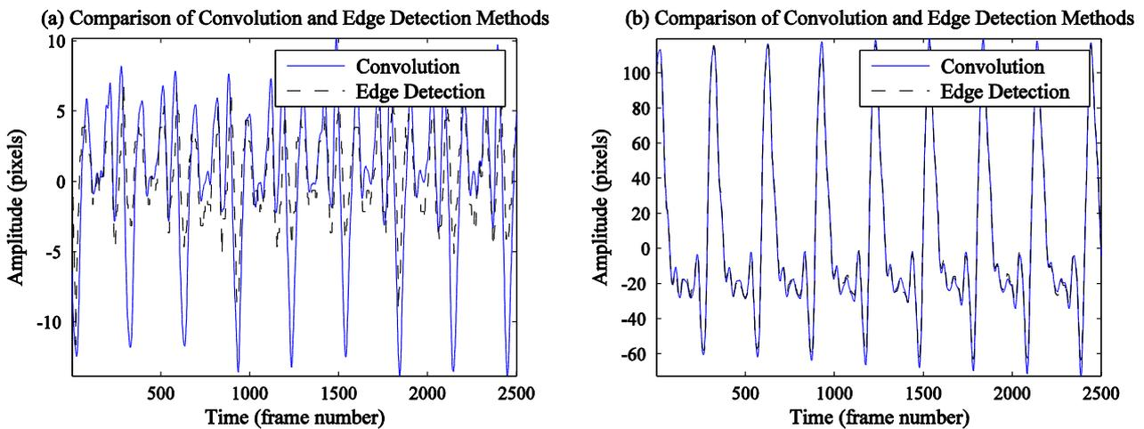
Figure 10: Comparison between vibration extraction methods for vertically plucked excitation
