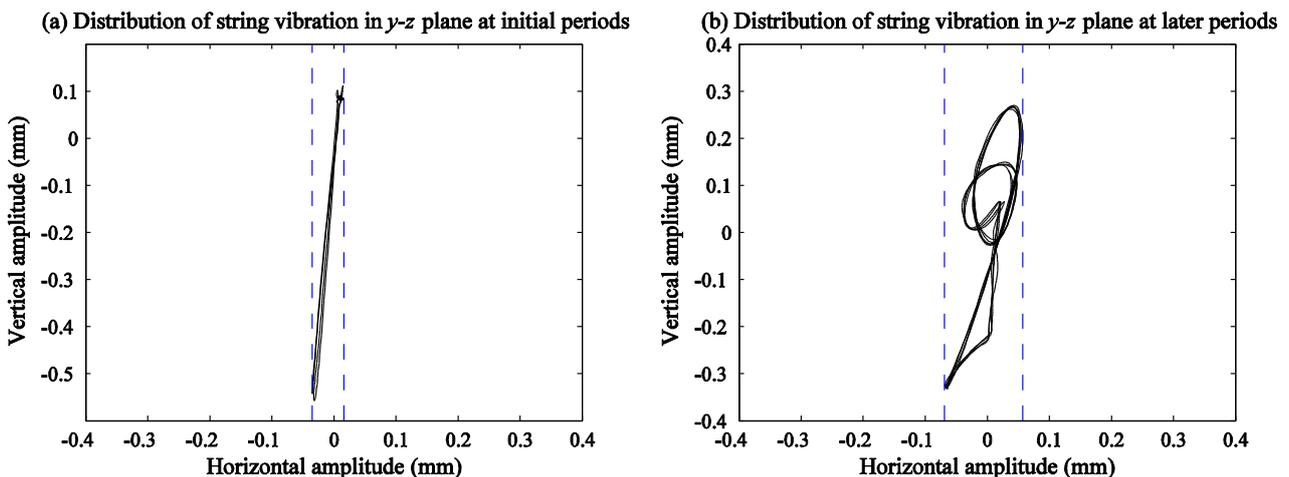
Figure 6: Distribution of string polarizations in  $y$ - $z$  plane for vertically plucked excitation at (a) the beginning of the oscillation and (b) after 0.8 seconds. Complement lines indicate the edges of the horizontal amplitude.
