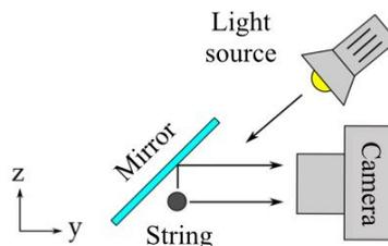
Figure 1: Scheme of the configuration with a single camera and mirror
