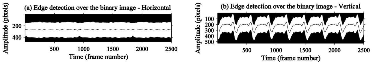
Figure 3: Waveforms of the extracted vibration signal using edge detection for (a) horizontal and (b) vertical polarizations in vertically plucked excitation plotted over the binary image
