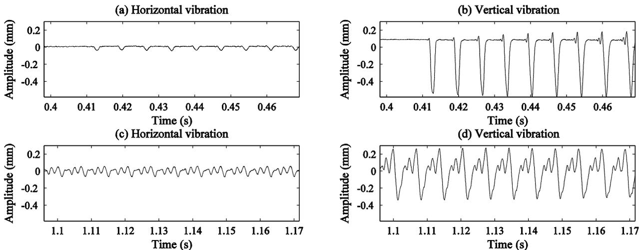
Figure 5: Waveforms of string polarizations in vertically plucked excitation. (a) and (b) are recorded at the beginning of the oscillation and (c) and (d) 0.8 s later.
