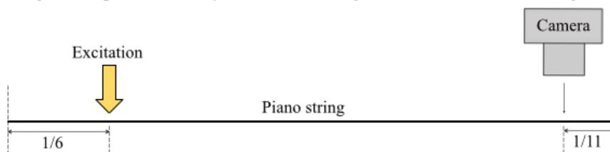
Figure 4: Scheme of the experiment set-up over a 1-meter piano string
