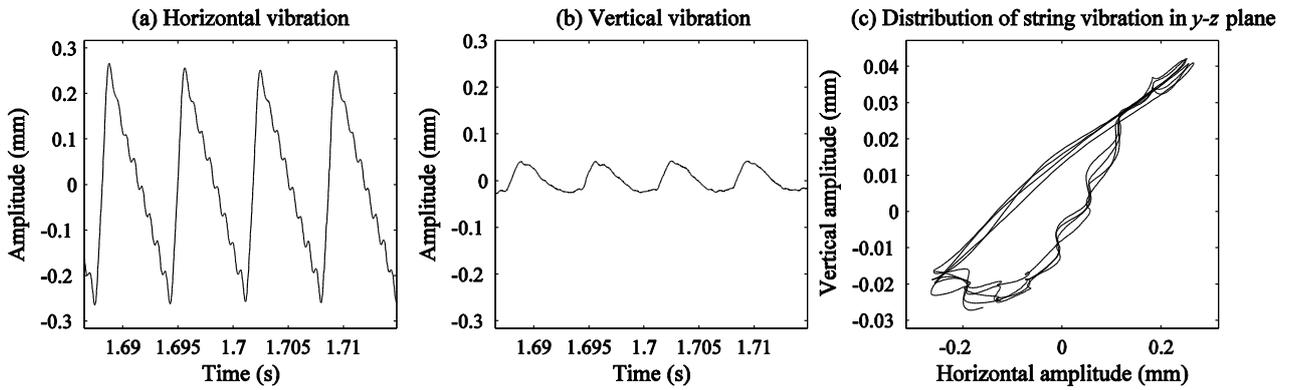
Figure 9: Waveforms of steady periods in horizontally bowed excitation for (a) horizontal and (b) vertical polarizations and (c) distribution of the string vibration in the  $y$ - $z$  plane
