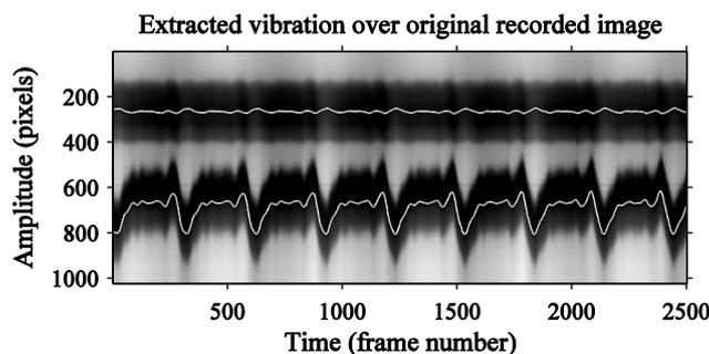
Figure 2: Waveforms of the extracted signal using convolution and peak detection for both polarizations in vertically plucked excitation plotted over the greyscale recorded image
