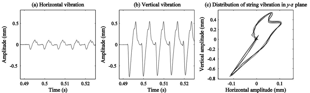
Figure 8: Waveforms of the first periods after vertically struck excitation for (a) horizontal and (b) vertical polarizations and (c) distribution of the vibration in the  $y$ - $z$  plane
