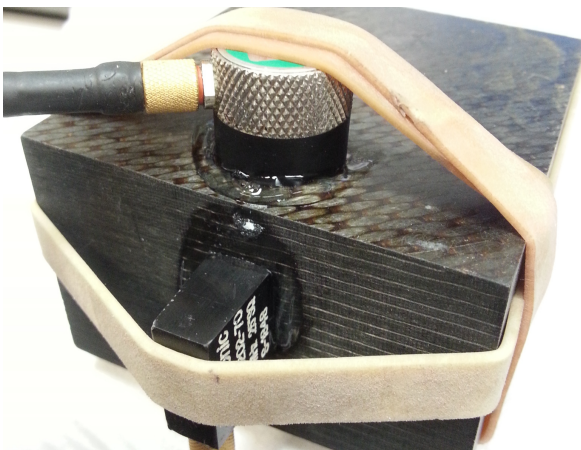
Figure 1: Carbon Fibre Reinforced Polymer (CFRP) block in the test configuration with transmitting transducer on side and receiving on top
