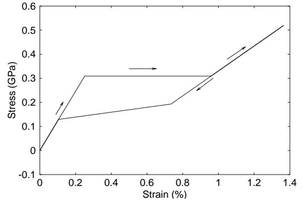
**Figure 2:** Local stress-strain behavior at a fixed point with full recovering of austenite.
