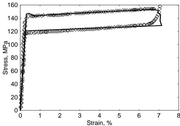
**Figure 3:** Stress-strain relation at the phase boundary: comparison with experimental data from Ref. [10]. Solid line corresponds to the numerical simulation.
