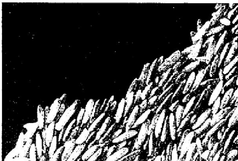
Fig. 8.21 A section of a rice pile confined between two glass plates. Notice how uneven the slope is on this fine scale. (Photo: Kim Christensen, University of Oslo.)
