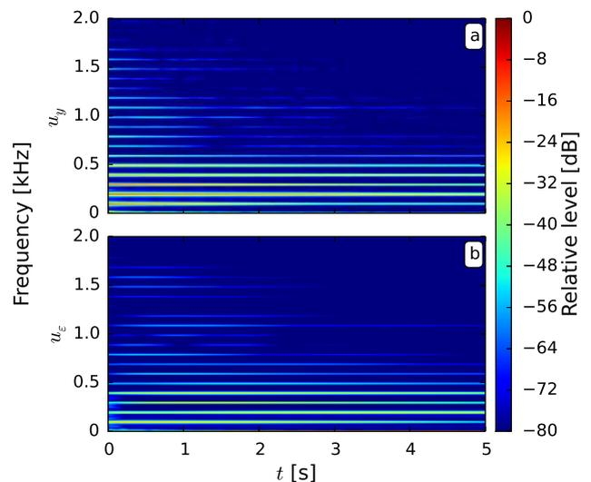
Figure 13: Spectrogram (a) of string vibration waveform that is excited in the horizontal direction, and (b) of a corresponding pickup signal waveform.
