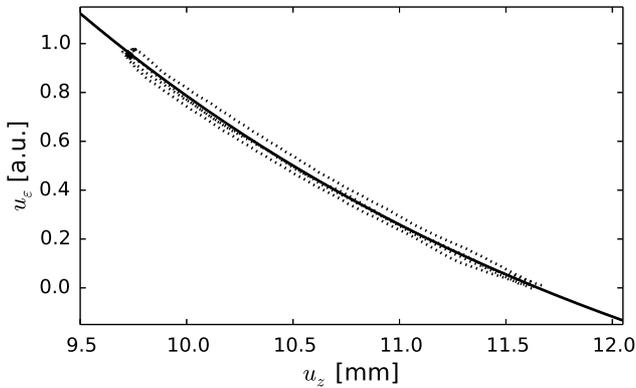
Figure 10: Mapping between the string's vertical displacements  $u_z$  and the corresponding pickup signal  $u_\epsilon$  for the first three periods. The measured data are shown by dotted line. The fitted exponential function in the form  $e^{-\alpha u_z}$  is shown by the solid line.
