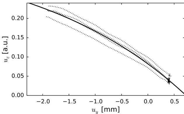
Figure 11: Mapping between the string's horizontal displacements  $u_y$  and the corresponding pickup signal  $u_\epsilon$  for the first three periods. Measurement data is shown by dotted line. Fitted polynomial function is shown by solid line.
