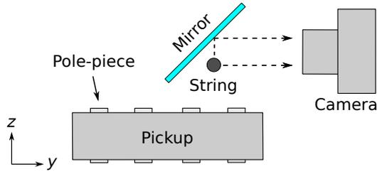
Figure 3: Optical string displacement measurement set-up that records the string vibration with respect to the vertical  $z$ -axis and horizontal  $y$ -axis simultaneously. A high speed line scan camera and a mirror that is placed under a  $45^\circ$  angle with respect to  $y$ -axis. Arrows with dashed lines indicate the direction of light propagation.
