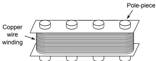
Figure 1: Magnetic pickup. The main components of the pickup are cylindrical permanent magnets called pole-pieces and the copper wire winding surrounding the magnets.
