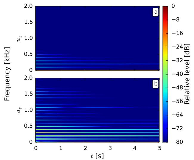
Figure 12: Spectrogram (a) of string vibration waveform that is excited in the vertical direction, and (b) of a corresponding pickup signal waveform.
