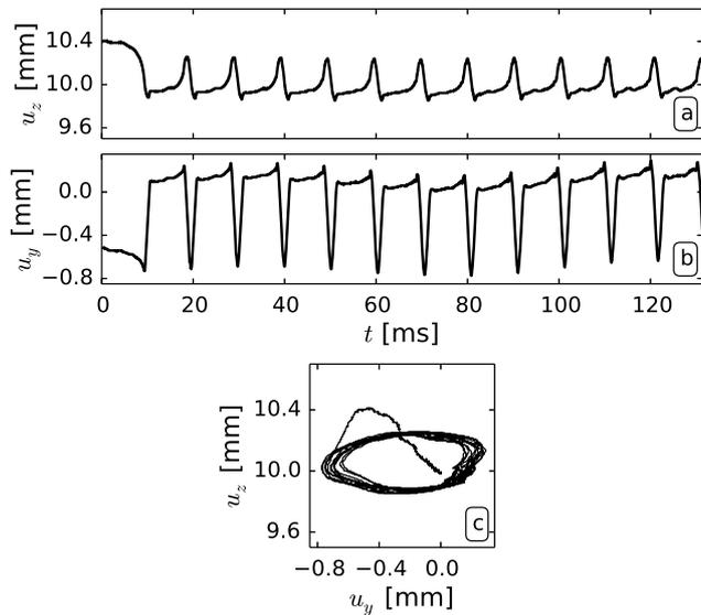
Figure 6: Vibration of the bass guitar string plucked with a plectrum. a) String displacement in the vertical direction. b) String displacement in the horizontal direction. c) String motion with respect to  $yz$ -plane.
