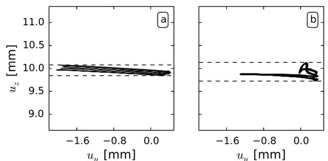
Figure 9: String vibration excited in the horizontal direction. a) The beginning of the vibration. b) Vibration 0.38 s later. Dashed lines indicate the amplitude extent in the vertical direction.
