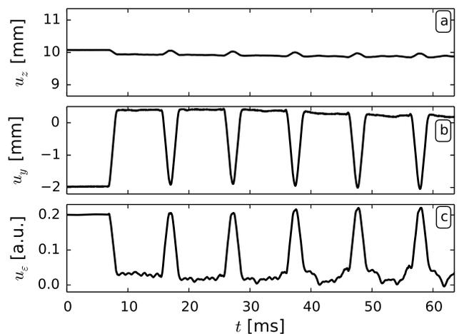
Figure 8: String vibration and a corresponding pickup signal. String is excited in the horizontal direction. a) String displacement in the vertical direction. b) String displacement in the horizontal direction. c) A normalized pickup signal.
