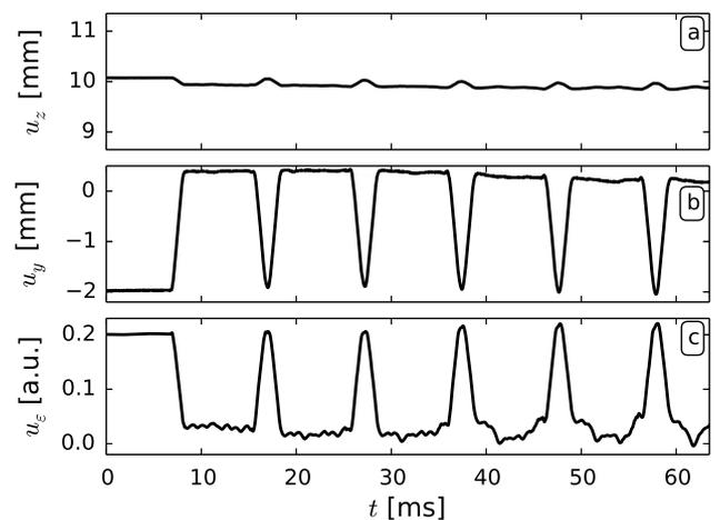
Figure 8: String vibration and a corresponding pickup signal. String is excited in the horizontal direction. a) String displacement in the vertical direction. b) String displacement in the horizontal direction. c) A normalized pickup signal.
