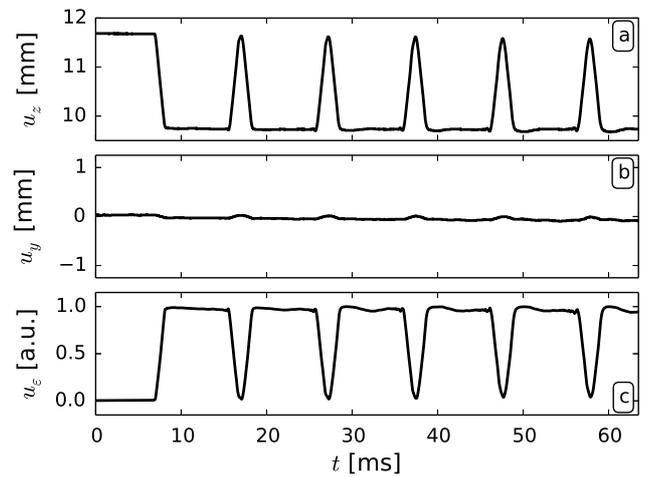
Figure 7: String vibration and a corresponding pickup signal. String is excited in the vertical direction. a) String displacement in the vertical direction. b) String displacement in the horizontal direction. c) A normalized pickup signal.
