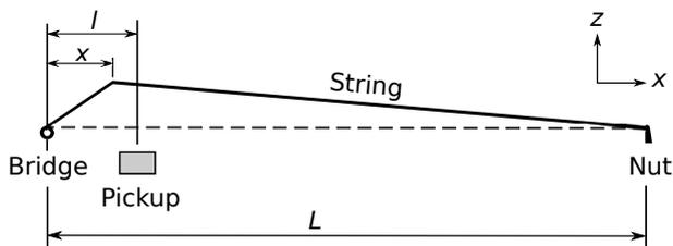
Figure 4: Triangular initial condition of the string, which is excited in the vertical direction. The string deflection maximum is located at  $x = 9.0$  cm. String speaking length  $L = 86.5$  cm. The location of the pickup is marked by  $l = 13.5$  cm. Dashed line shows the form and the position of the string at rest.
