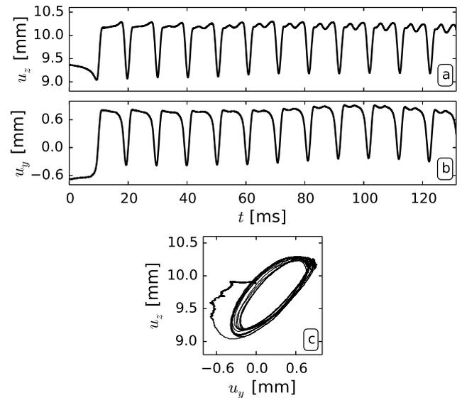
Figure 5: Vibration of the bass guitar string plucked with an index finger. a) String displacement in the vertical direction. b) String displacement in the horizontal direction. c) String motion with respect to  $yz$ -plane.
