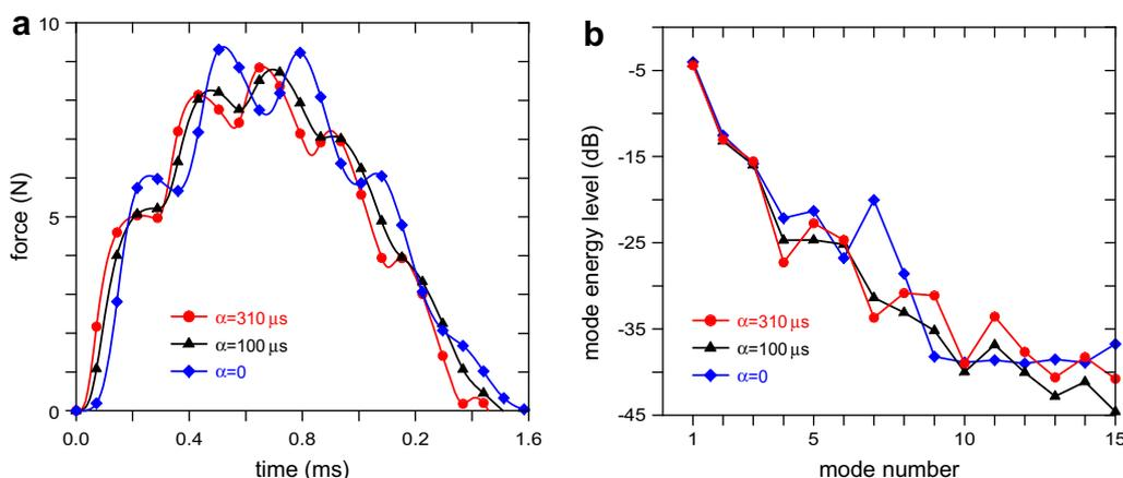
Fig. 3. Force histories (a) and spectral envelopes (b) for string  $n = 49$ . Varying retarded time parameter  $\alpha$  with fixed compliance nonlinearity exponent  $p = 4.43$ , and static hammer stiffness  $Q_0 = 1660$  N/mm<sup>p</sup>.
