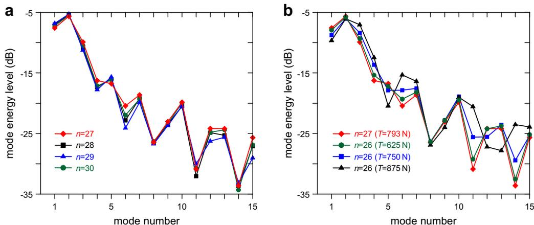
Fig. 2. Comparison of spectral envelopes. (a) All strings are terminated on treble bridge and (b) for string  $n = 27$  terminated on treble bridge, and for various tension  $T$  of string  $n = 26$  terminated on bass bridge.
