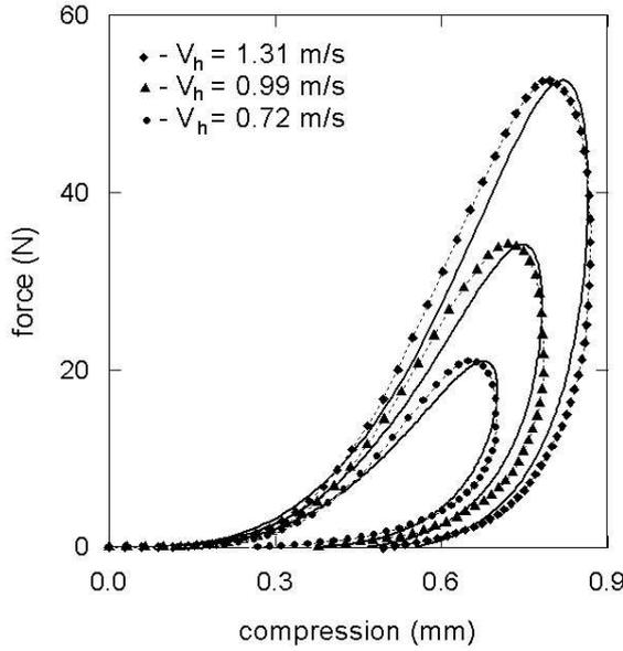
**FIGURE 1.** The measured (various signs) and simulated (solid lines) force-compression characteristics of the piano hammer for the various hammer velocity.
