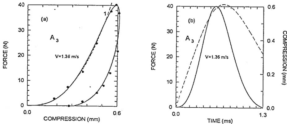
Fig.1. Dynamical features of hysteretic hammer. (a) Solid circles denote the experimental data points (Ref. 7); solid line is the simulated force-compression characteristic for medium hammer, identical to Fig.1(b) in Ref.10; dashed line 1 is approximation of the loading part of the hysteretic curve ( $F_0 = 175 N/mm^p$ ,  $p = 2.5$ ). (b) Force-time (solid line) and compression-time (dashed line) characteristics of the same hammer.
