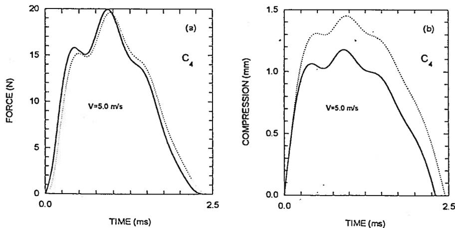
Fig.3. Interaction of hammers with initial velocity  $V = 5.0\text{m/s}$  with a flexible string, using the same hammer's parameters, as in Fig.2. (a) Force histories. (b) Compression histories; for hysteretic (solid line) and nonhysteretic (dotted line) hammers.
