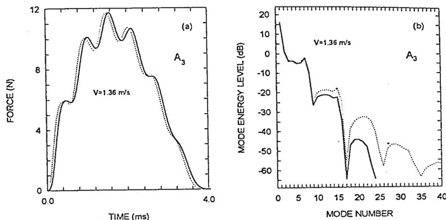
Fig.5. Force histories (a), and spectra envelopes (b) for nonlinear medium hammer  $A_3$  and flexible string with parameters presented in Ref.10. Solid lines represent the results for hysteretic hammer, using  $\epsilon = 0.956$ ,  $\tau_0 = 7\mu s$ ,  $p = 3.3$ ,  $F_0 = 3580 N/mm^p$ , dotted lines for nonhysteretic hammer, using  $F_0 = 175 N/mm^p$ ,  $p = 2.5$
