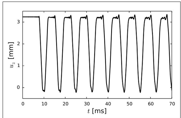
Figure 10. Vibration of a stiff steel string in the vertical direction showing the dispersion effect.
