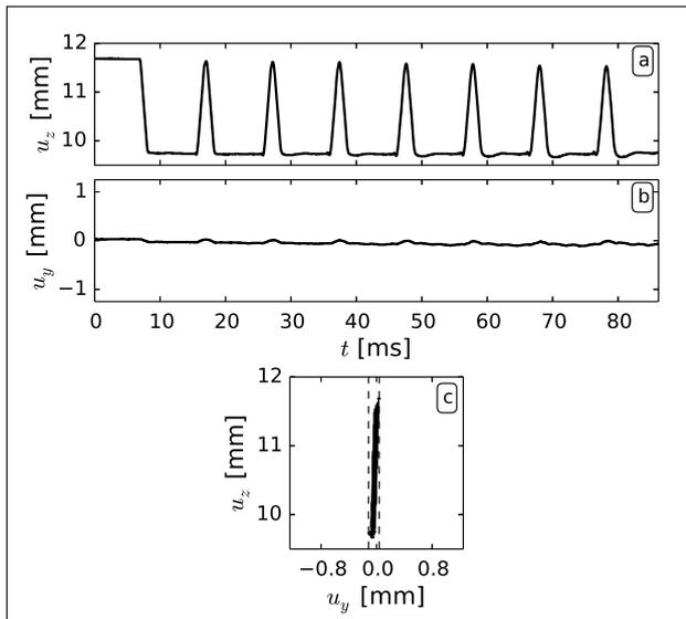
Figure 8. String vibration right after the string was excited in the vertical direction. a) String displacement in the vertical direction. b) String displacement in the horizontal direction. c) String motion with respect to  $yz$ -plane. Dashed lines indicate the amplitude extent in the horizontal direction.
