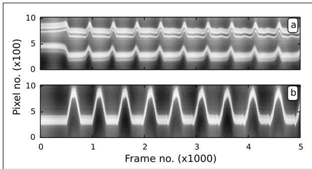
Figure 3. Image files as recorded by the line scan camera under different lighting conditions. a) The bass guitar string motion as recorded by using the camera and a mirror set-up. Top half of the image shows the displacement  $u_z$  and bottom half the  $u_y$ . b) The piano string's vertical displacement  $u_z$  as recorded by single camera.
