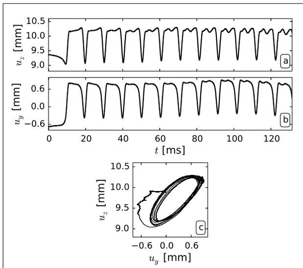
Figure 6. Vibration of the bass guitar string plucked with an index finger. a) String displacement in the vertical direction. b) String displacement in the horizontal direction. c) String motion with respect to  $yz$ -plane.
