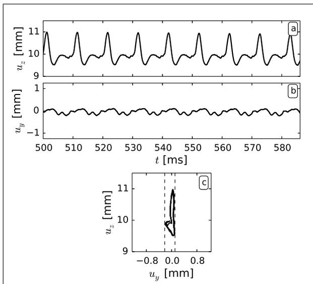
Figure 9. String vibration 0.5 s after excitation in the vertical direction. a) String displacement in the vertical direction. b) String displacement in the horizontal direction. c) String motion with respect to  $yz$ -plane. Dashed lines indicate the amplitude extent in the horizontal direction.
