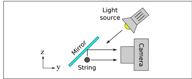
Figure 2. Single camera and a mirror set-up. Arrows indicate the direction of light propagation.
