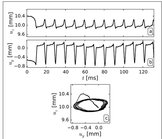
Figure 7. Vibration of the bass guitar string plucked with a plectrum. a) String displacement in the vertical direction. b) String displacement in the horizontal direction. c) String motion with respect to  $yz$ -plane.
