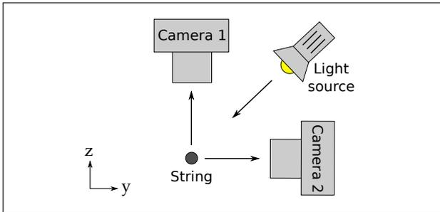
Figure 1. Two camera set-up. Arrows indicate the direction of light propagation.
