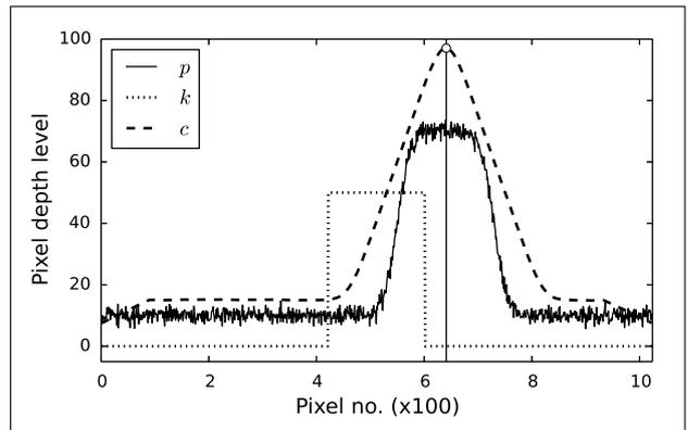
Figure 4. The correlation of a single frame. Solid line  $p$  shows the recorded image profile. The correlation kernel  $k$  is shown by dotted line. The correlated frame profile  $c$  is shown by dashed line. Vertical line show the position of the image region that is most similar to selected kernel profile. Higher depth levels correspond to image regions with higher illumination.
