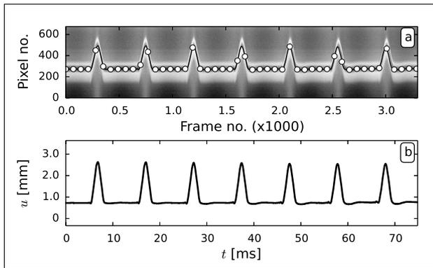
Figure 5. Vibration of a bass guitar G string, with a triangular initial condition. a) The recorded image. Displacement of the maximum of the correlated frame  $c$  relative to the image is shown by solid line marked by bullets. b) The corresponding extracted and calibrated displacement  $u(t)$ .
