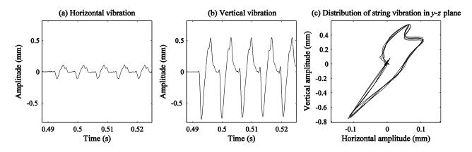
Figure 8: Waveforms of the first periods after vertically struck excitation for (a) horizontal and (b) vertical polarizations and (c) distribution of the vibration in the *y*-*z* plane
