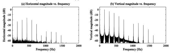
Figure 7: Spectrum of string vibration in vertically plucked excitation for (a) vertical and (b) horizontal polarizations
