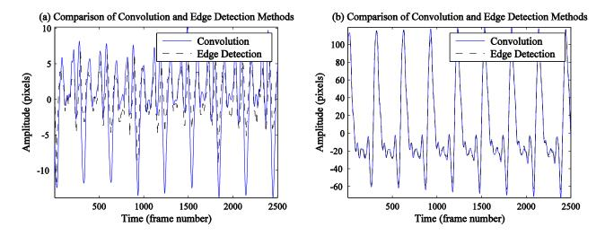
Figure 10: Comparison between vibration extraction methods for vertically plucked excitation
