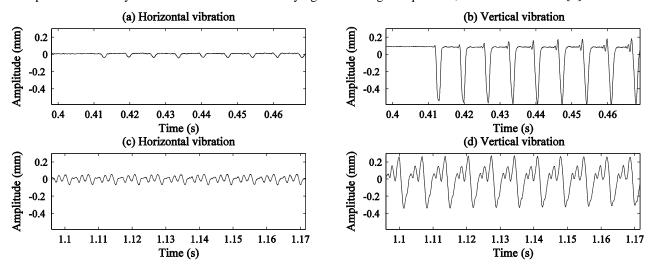
Figure 5: Waveforms of string polarizations in vertically plucked excitation. (a) and (b) are recorded at the beginning of the oscillation and (c) and (d) 0.8 s later.
