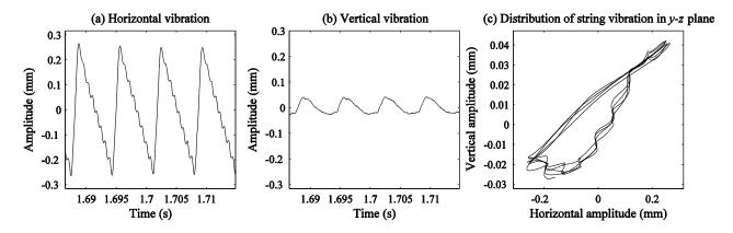
Figure 9: Waveforms of steady periods in horizontally bowed excitation for (a) horizontal and (b) vertical polarizations and (c) distribution of the string vibration in the *y*-*z* plane
