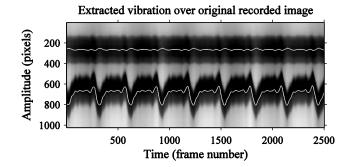
Figure 2: Waveforms of the extracted signal using convolution and peak detection for both polarizations in vertically plucked excitation plotted over the greyscale recorded image
