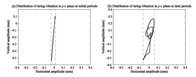
Figure 6: Distribution of string polarizations in *y*-*z* plane for vertically plucked excitation at (a) the beginning of the oscillation and (b) after 0.8 seconds. Complement lines indicate the edges of the horizontal amplitude.
