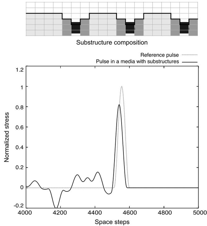
Fig. 2. Pulse shape in “hard-intermediate-soft-intermediate-hard” double structure laminate.
