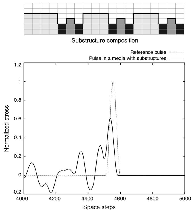
Fig. 1. Pulse shape in “hard-soft-intermediate-soft-hard” double structure laminate.
