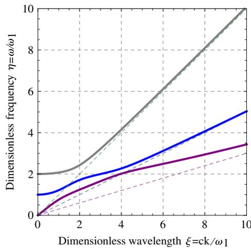
Fig. 3. Dispersion curves of Eq. (40) for  $\gamma_{A1} = \gamma_{A2} = 0.4$ ,  $\gamma_1 = 0.5$ ,  $\gamma_2 = 0.3$ ,  $\eta_2 = 2$ : solid lines — concurrent microstructure model, dashed lines — asymptotes to dispersion curves.
