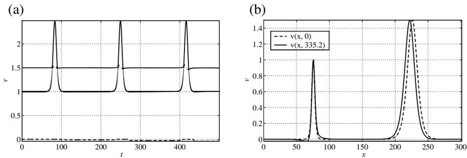
**Fig. 2.** Head-on collision of solitary waves with nonequal amplitudes. (a) Waveprofile minima and maxima against time. (b) The initial waveprofile and the waveprofile after two interactions at  $t = 335.2$ .
